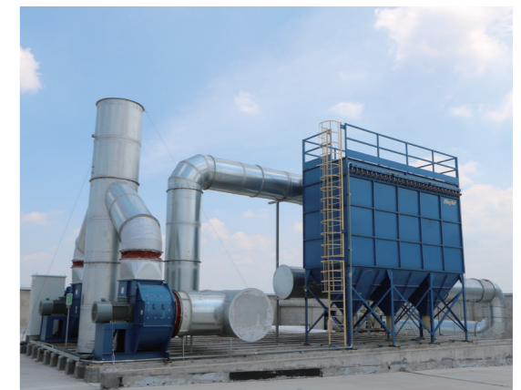
BAG DUST COLLECTOR Applied in semiconductor packaging and testing dust removal
