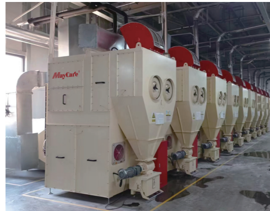
HORIZONTAL INSERT-TYPE SINGLE MACHINE Applied in lithium battery cell production lines
