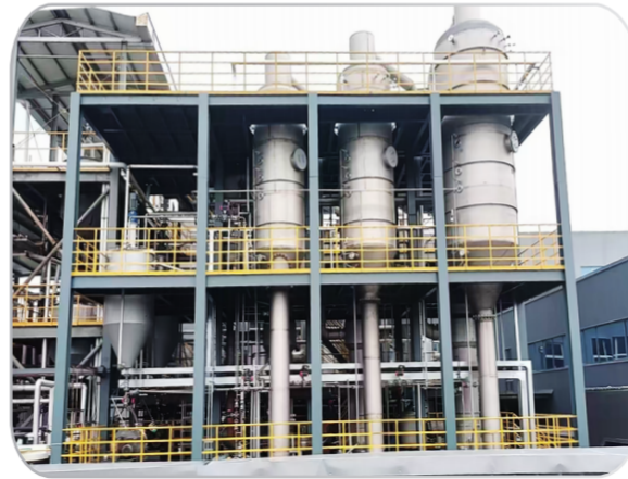
三效强制循环结晶器 Three-effect Forced Circulation Crystallization evaporator
