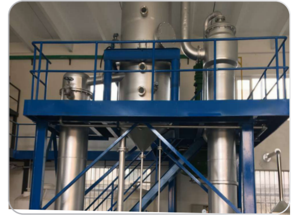
单效强制循环结晶器 Single-effect Forced Circulation Crystallization evaporator
