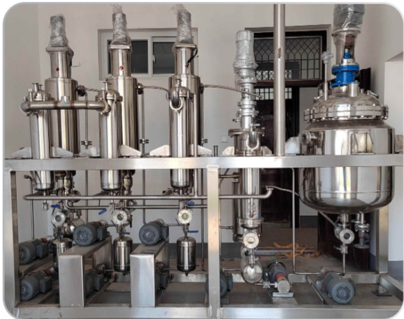
刮板式薄膜蒸发器 Scraper Type Film Evaporator
